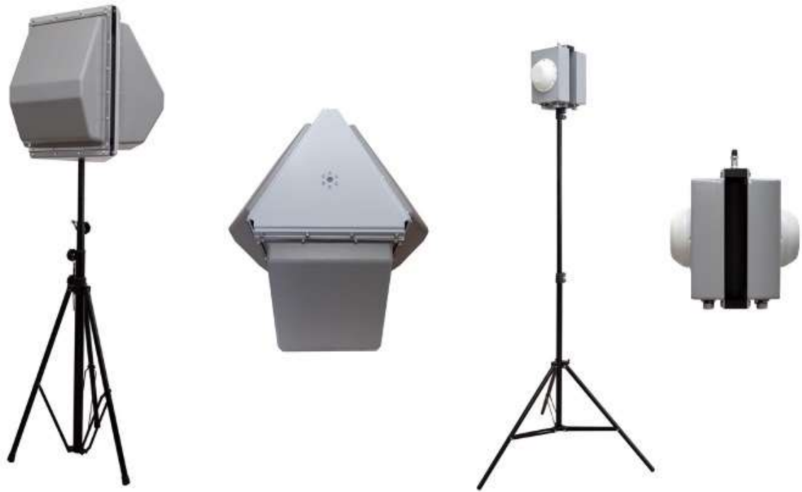
Fig. 1. Mock-up of the receiver (left) and transmitter (right)
